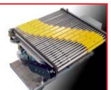
(1" diam.) on which plastic slats slides from one side to the other. The switching is done by a metallic finger pneumatically actuated which direct the slats into a guiding track.
